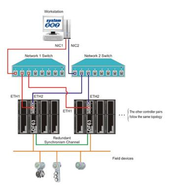
Basic architecture for DFI302 controllers with two Ethernet ports
